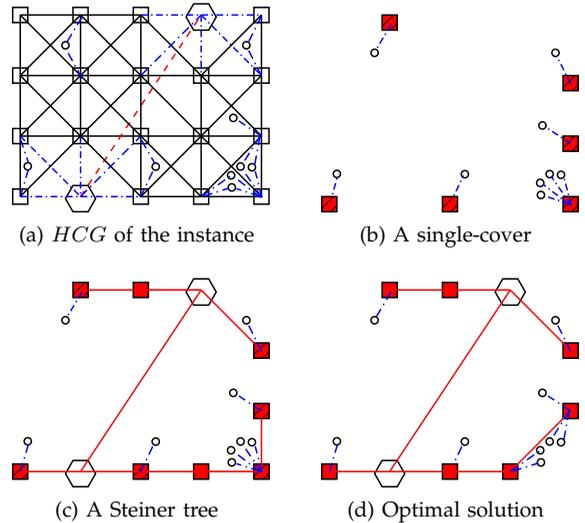
Fig. 2: (a) The  $HCG$  for 2 BSs (hexagons), 9 SNs (circles), and 18 candidate RN locations (squares). (b) A feasible solution to SCP. (c) The resulting 1CSC, which uses 8 RNs. (d) The optimal solution, which uses 7 RNs.
